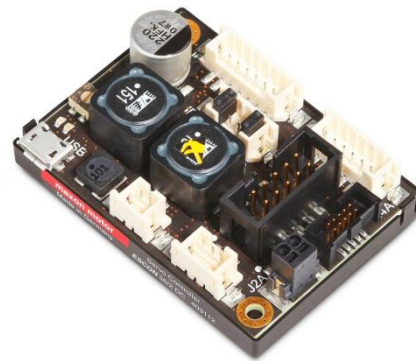
ESCON 36/2 DC – digital servo controller for DC motors up to 72 W, dimensions 55 x 40 x 16.1 mm
